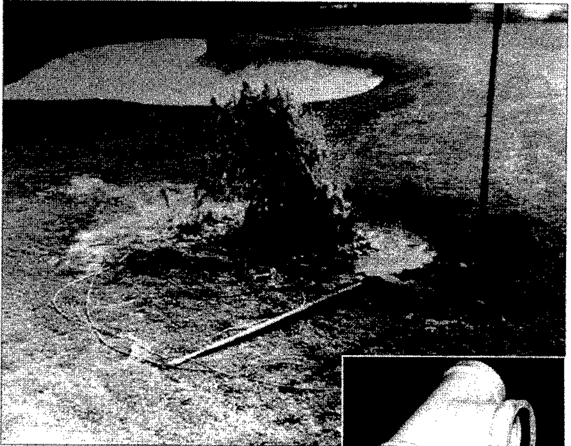
Above: Failed PVC fittings produce scenes like this at golf courses all over the country. Repeated replacement can be avoided by using ductile-iron fittings on any full-dimension tee or mainline change of direction that is three inches or larger. Photos courtesy: The Harrington Corporation.
