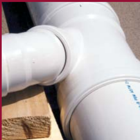
Figure 4 Close-up photographs of the fittings when over-stressed.
